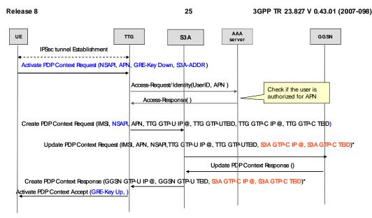
\*Depending on operator's configuration with regards to the user plane path rules, the user plane may go through the S3A. In this case, the S3A sends an Update PDP context request / Create PDP context response with its own TEID and IP addresses for control and user planes.
