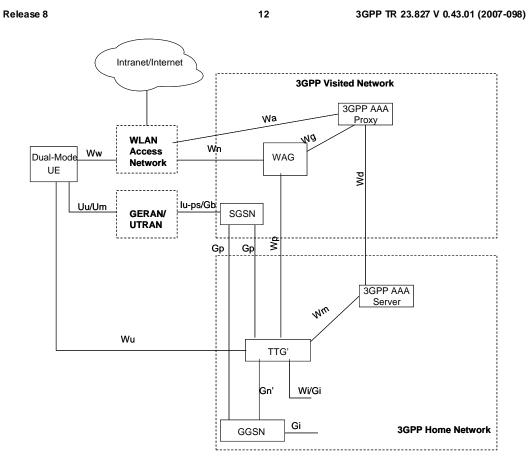
Figure 6.2.2 : Roaming Architecture for I-WLAN Mobility
