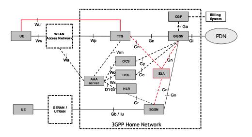
Figu re 6.2.8 Non-Roaming Reference model for I-W LAN/3GPP Mobility
