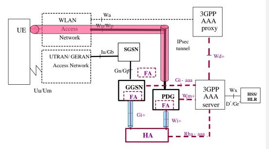
Figure A.4: Use of MIPv4 with FA-CoA for GPRS-WLAN mobility
