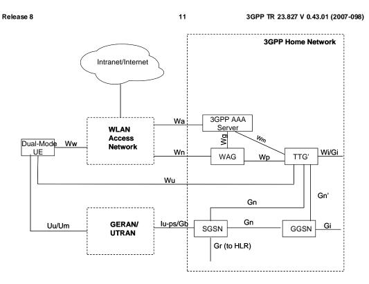
Figure 6.2.1 : Non-Roaming Architecture for I-WLAN Mobility
