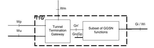
Figure 6.2.4 : TTG' implementation re-using GGSN functionality
