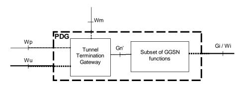
Figure 6.2.3 : PDG implementation re-using GGSN functionality (from 23.234)
