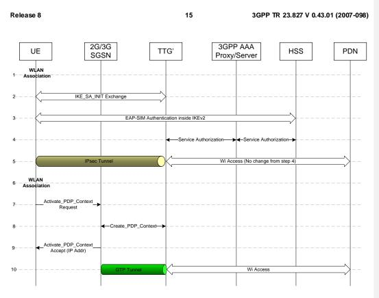
Figure 6.2.5 Handover from pre-SAE 3GPP to I-WLAN (Wi services)
