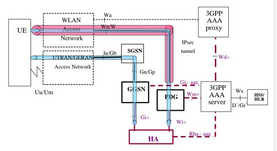
Depicted in Figure A.5 is the application of Mobile Ipv6 as a solution for inter-system mobility. The same figure also applies to the use of MIPv4 with collocated Care-of-Addresses (co-CoA).
