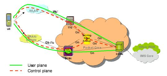
Figure 6.2.9 Handover mechanism for I-WLAN/3GPP Mobility
