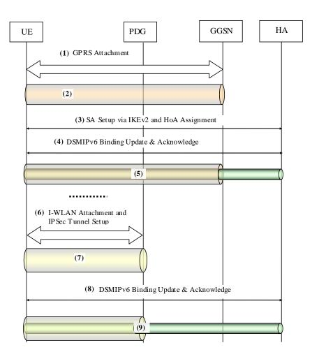
Figure 6.2.19 Information Flow for Initial Attach in GPRS and subsequent Handover to I-WLAN (non-roaming case)
