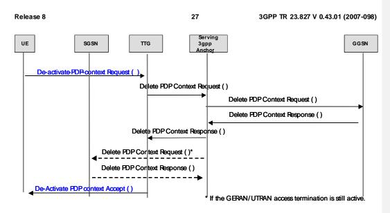
Figure 6.2.15 PDP context de-activation on the WLAN side
